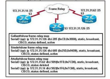
A: The Gallant router has the wrong LMI type configured.
